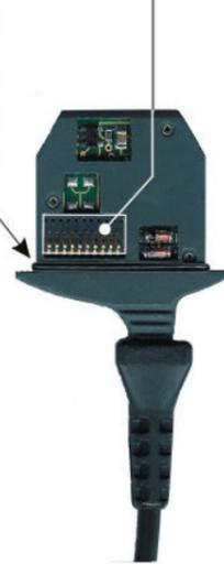
Connection pins to the instrument (do not damage, keep clean)
